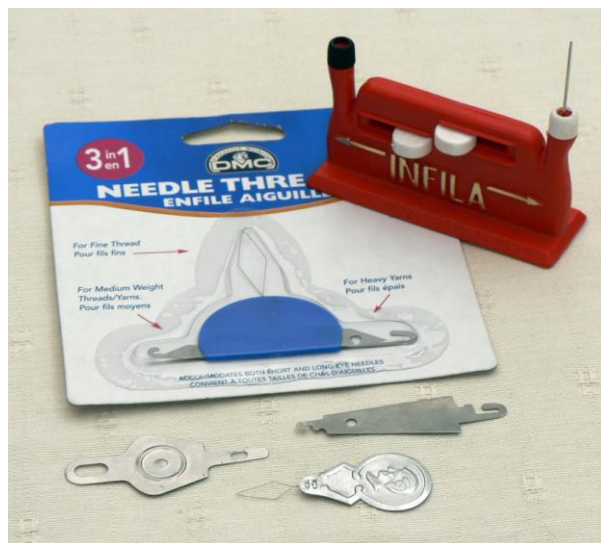
Fig.1 Needle threaders range from fine wire for floss to more substantial threaders
